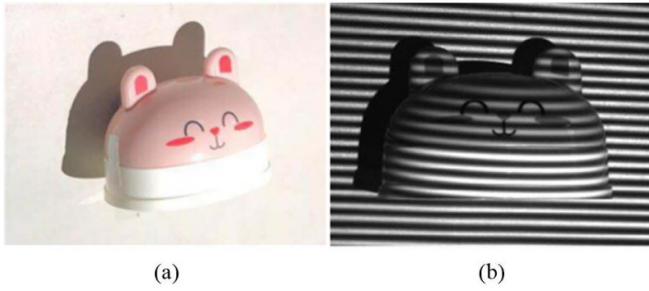
Figure 1. The object used in the experiment. (a) The cartoon face object; (b) the captured fringe pattern of the object to be measured.
